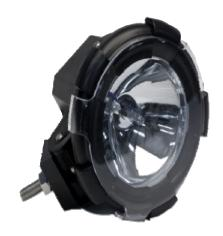
These lights have internal Ballast are 35 W HID and come in either Spot or Flood Beam.
